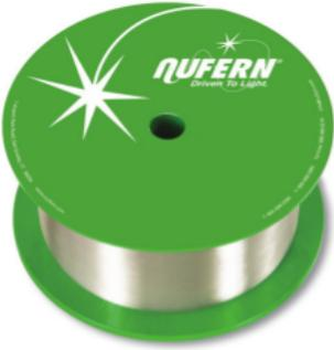
Nufern's specialty multimode step-index fibers are designed for compatibility with the majority of fiber-coupled, bar and stack diode-laser packages and support the diode laser power delivery market. These power delivery fibers are available in 200/220 and 200/240 core/clad ratios in low and high NA versions. Other fiber diameters are available upon request.
